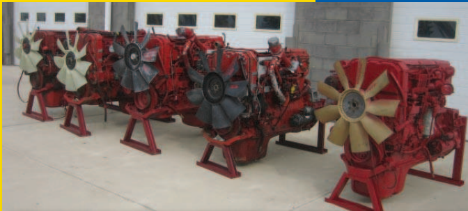
Several ISX Cummins Engines
