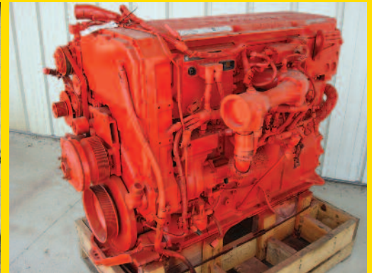
2002 CUMMINS ISX 500HP CPL 8285, S/N#14031552, EGR, GOOD RUNNER
