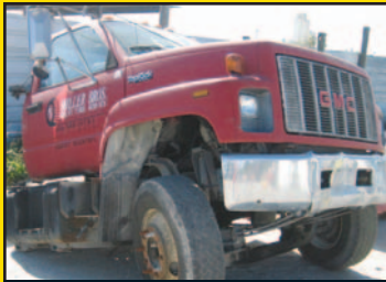
1994 Chevrolet TopKick Cab Clip CATERPILLAR 3116 250 HP Fuller 6 Speed Transmission
