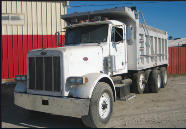
1993 Peterbilt Dump Truck 3306 Caterpillar, Fuller RTO 8 Speed LL, Eaton DS 461 P, 46,000 Hendrickson Suspension
